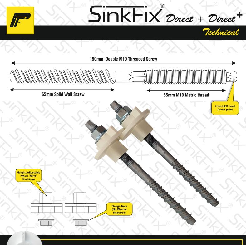
SinkFix® has specially designed nylon bushings that have four positioning points which can raise the wash basin for fine horizontal adjustment on each side by up to 5mm.
